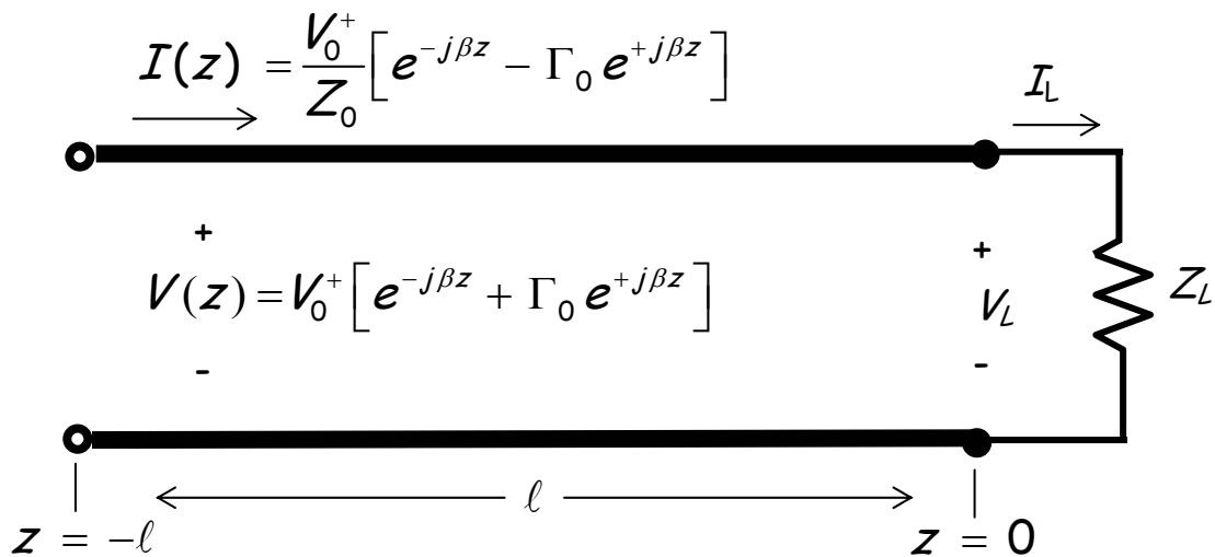
The result is that electromagnetic energy flows along the transmission line at a given rate (i.e., **power**).
