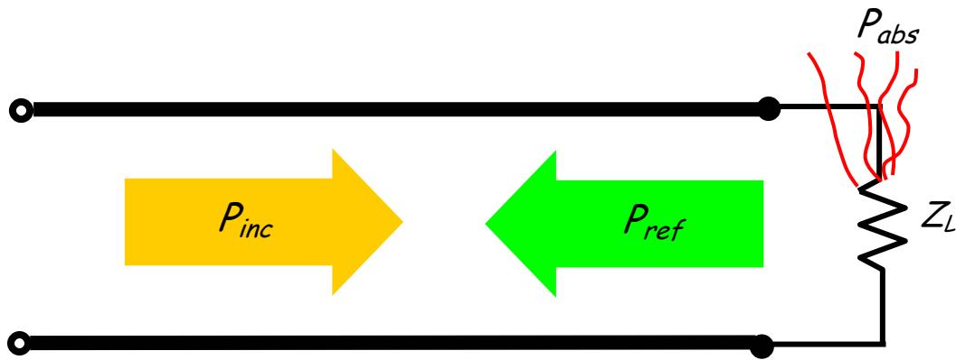
Note that if  $|\Gamma_L|^2 = 1$ , then  $P_{inc} = P_{ref}$ , and therefore **no power is absorbed by the load**.
